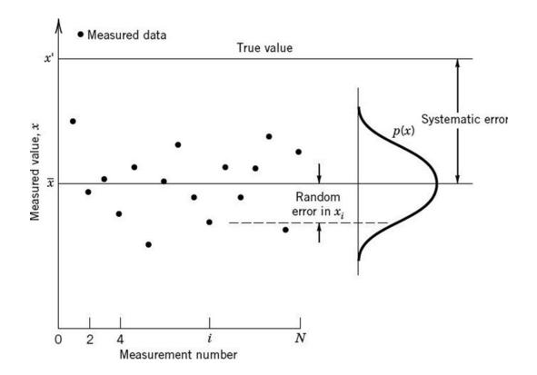
Figure 3.1 Distribution of errors upon repeated measurement [3]
